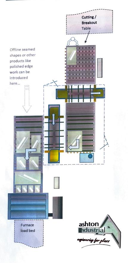
Depicted with standard endloading roller conveyor with integrated pop-up castors and side datum guide wheels.
