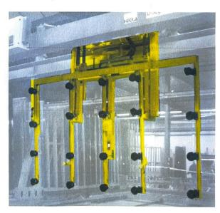
Single glass sheets - float glass as well as laminated glass - are picked up automatically from their storage position and transferred to a tilting table for feeding a cutting line.
