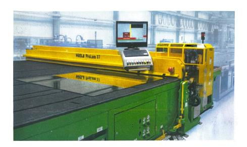
The cutting machine ProLam combines the process steps cutting - break out - separating
