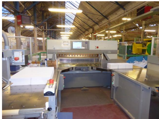
Polar guillotine model 155XT, number 7921103, with light guarding, air float table, power back fence, year 2010, auto stacker and de stacker.
